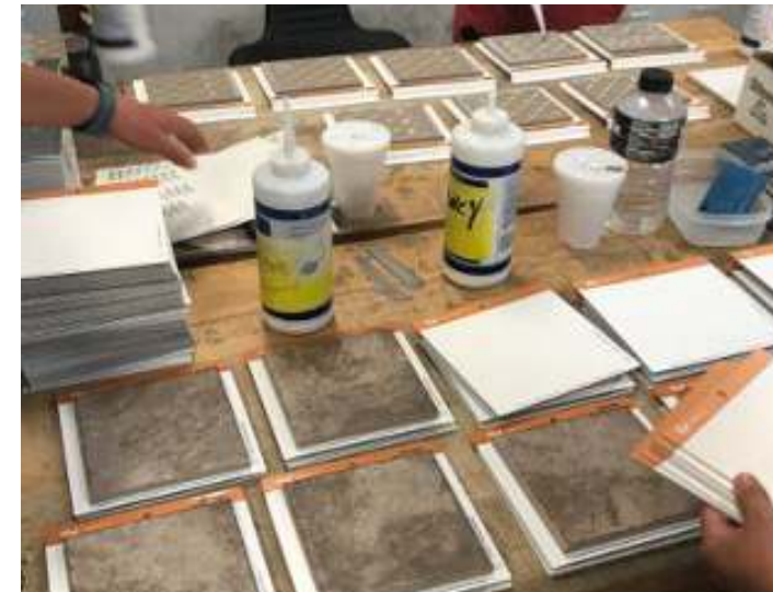
POOLCORP's new tile assembly process eliminated strain on employees' hands and backs while resulting in a 91% increase in throughput.
